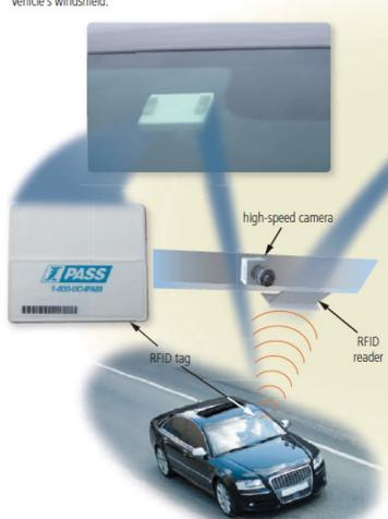
Step 2 As the vehicle approaches the tollbooth, the RFID reader in the tollbooth sends a radio wave that activates the windshield-mounted RFID tag. The activated tag sends vehicle information to the RFID reader.
