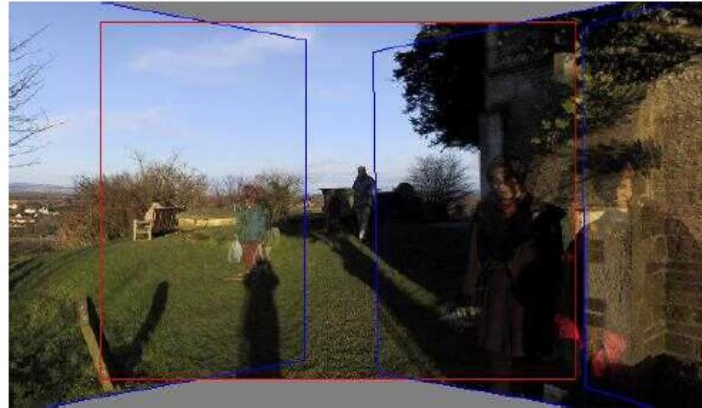
Figure 8.13 Validation of image matches by direct pixel error comparison can fail when the scene contains moving objects (Uyttendaele, Eden, and Szeliski 2001) © 2001 IEEE.
