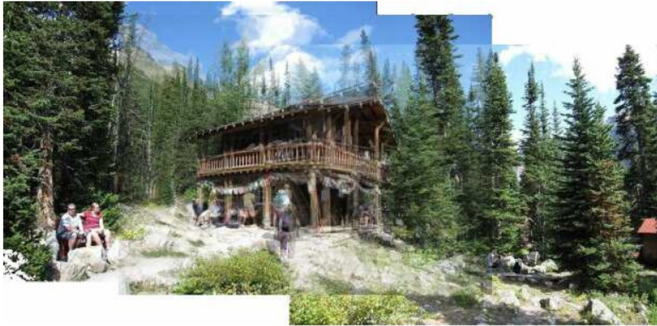
Figure 8.3 A simple panograph consisting of three images automatically aligned with a translational model and then averaged together.
