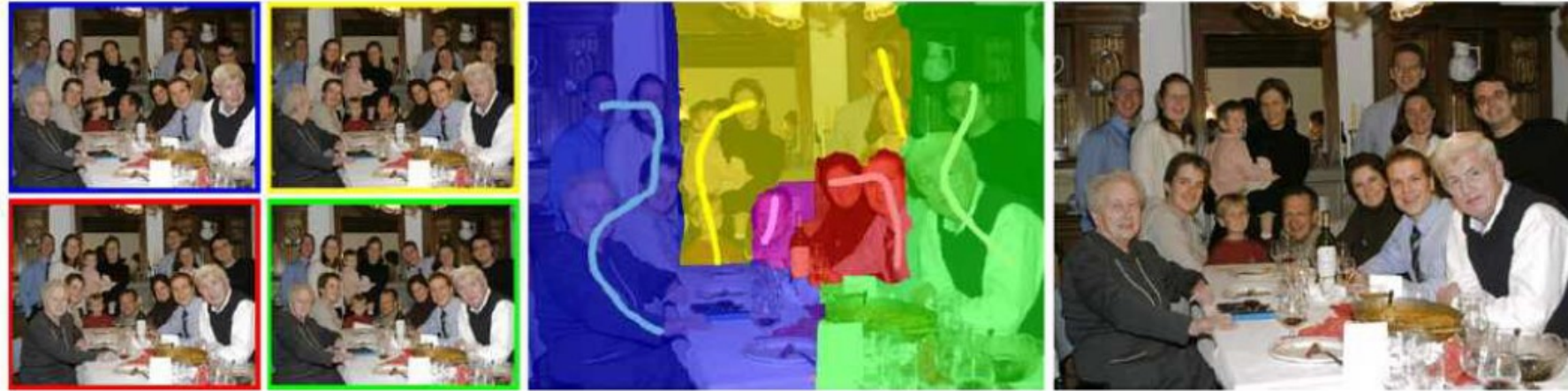
Figure 8.16 Photomontage (Agarwala, Dontcheva et al. 2004) © 2004 ACM. From a set of five source images (of which four are shown on the left), Photomontage quickly creates a composite family portrait in which everyone is smiling and looking at the camera (right). Users simply flip through the stack and coarsely draw strokes using the designated source image objective over the people they wish to add to the composite. The user-applied strokes and computed regions (middle) are color-coded by the borders of the source images on the left.
